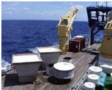
Two wind profiler radars (large white boxes) on the deck of the R/V Menai. One is a MRF and the other is a RAS. There is also a RAS and an S-band vertically pointing radar (the arm above).
