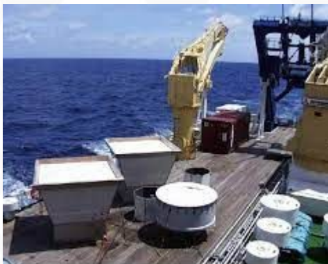
Two wind profiler radars (large white boxes) on the deck of the R/V Menai. One is a 300W and the other is a 100W. There is also a RASD system and an S-band vertically pointing radar (the arm at the end).
