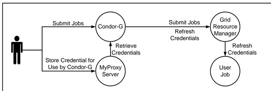
For example, a user can submit a long-running task to a job broker like Condor-G and authorize the broker to use MyProxy to renew credentials. If the job queues or runs longer than the lifetime of the credentials, the broker can authenticate to MyProxy and retrieve new credentials for the job, so the job can continue accessing Grid resources during its run.
